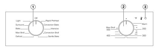
Mode selector To select oven modes ③ Temperature indicator light Indicates that the oven is heating
