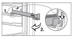
Hook the FlexiClip runner onto the front of the top rail of a side runner (1.) and then hold it at an angle in towards the middle of the oven compartment (2.).
