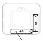
Insert fresh alkaline AA batteries and reinstall thermostat.
