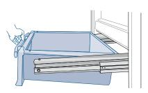
to remove the drawer, unscrew the locking nuts and remove the drawer
