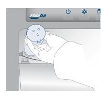
The filter is located inside the refrigerator compartment, near the door hinge, protected by a flap door. Prior to change the filter switch off the Ice Maker by pressing the IceMaker button. Then enter the Fhiaba Access Menu and set "Manual Clean" function. At the end of the cleaning cycle remove the water from the ice tray and wipe it dry.
