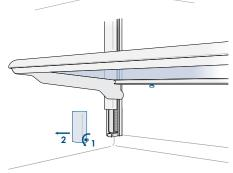
• to remove a shelf it is necessary to first remove the end parts of the guides (unscrew the locking nut), slide it downwards and remove it.
