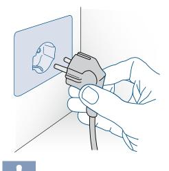
The appliance is equipped with a Schuko type 16A plug and must be connected to the electrical power supply through a corresponding Schuko socket.
